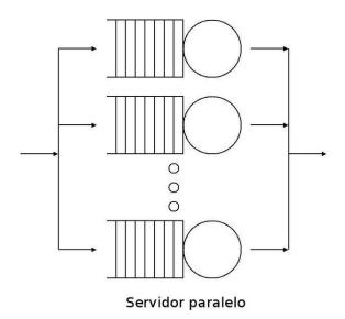
Queue networks are systems in which single queues are connected by a routing network. In this image servers are represented by circles, queues by a series of retangles and the routing network by arrows. In the study of queue networks one typically tries to obtain the equilibrium distribution of the network, although in many applications the study of the transient state is fundamental.
