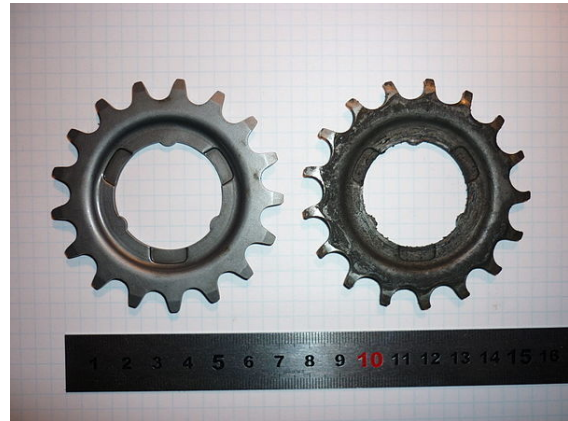
Rear sprocket for a bicycle where the left is unused and the right has obvious wear from clockwise rotation.
