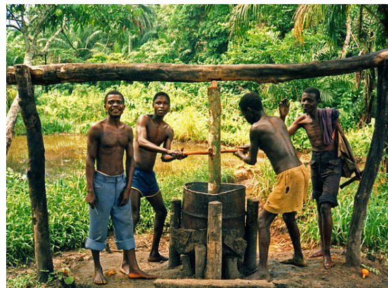
A village palm oil press “malaxeur” in Bandundu, Democratic Republic of the Congo
