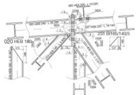
Typical detail of a steel truss, which is considered as a revolute joint
