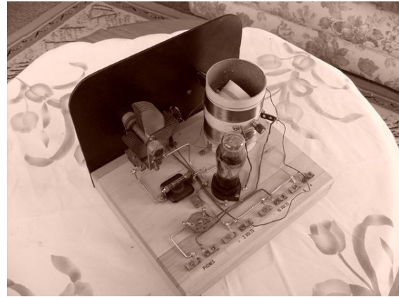
A vintage style regenerative radio receiver. Due to the controlled use of positive feedback, sufficient amplification can be derived from a single vacuum tube or valve (centre).
